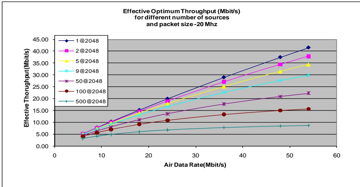
The above graph is good only as a marketing tool, since we manipulated the parameters to get the maximum result. We considered packets sent only in one direction, adjusted the timings for a very short link (few meters), no interference was considered and the transmitted packets were maximized to the highest size of 2048 Bytes.
