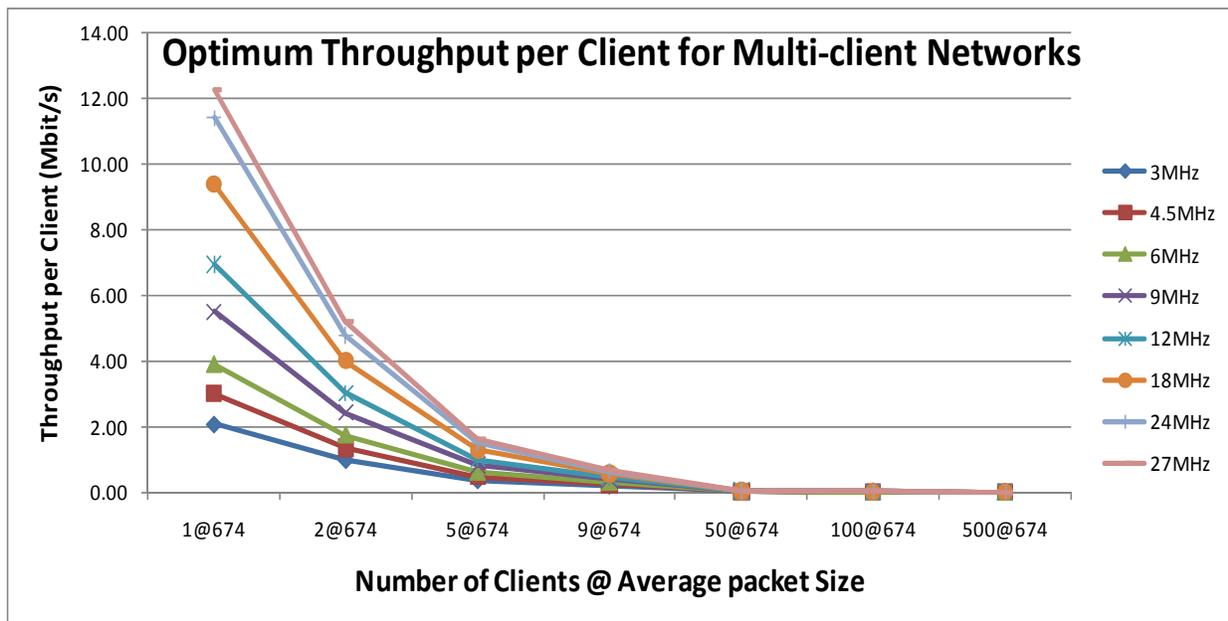
The above throughputs represent the maximum throughput in the air. They have to be discounted by the FEC (Forward Error Code) which will yield between 80 and 50% of the above throughput, plus the wireless protocol (MAC) which will consume another 5%. The best actual throughput available for the applications is between 75% and 45% of the one shown in the graphs. Summarizing:
