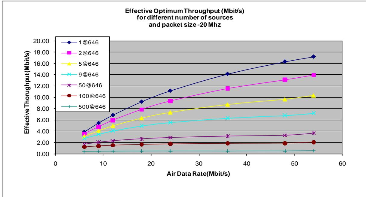
Furthermore, it should be noted that a 20 MHz channel compromises the frequency reuse in the 4.9 GHz band and will render a network non expandable. This bandwidth should be only be used in specific point to point connection, with highly directional antennas.
